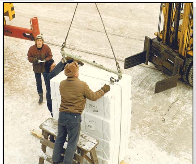
Cranston UNI-LIFT hooks shown in a typical operation with a spreader bar.
