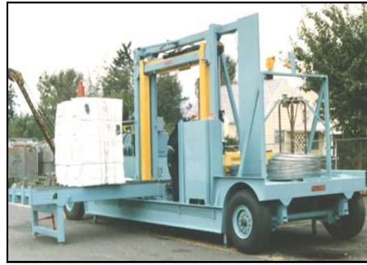
"Portatizer" Econotizer and conveyors on trailer.
