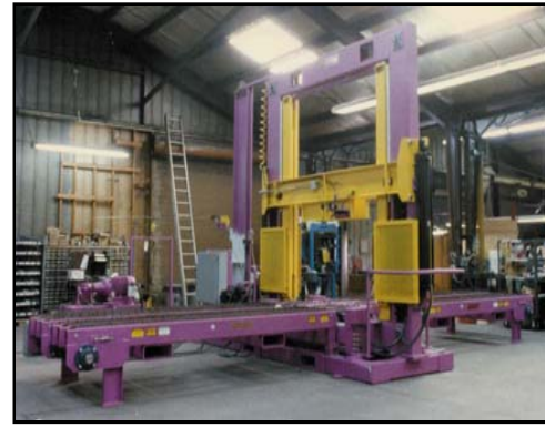
967 Unitizer with portability kit and conveyors.
