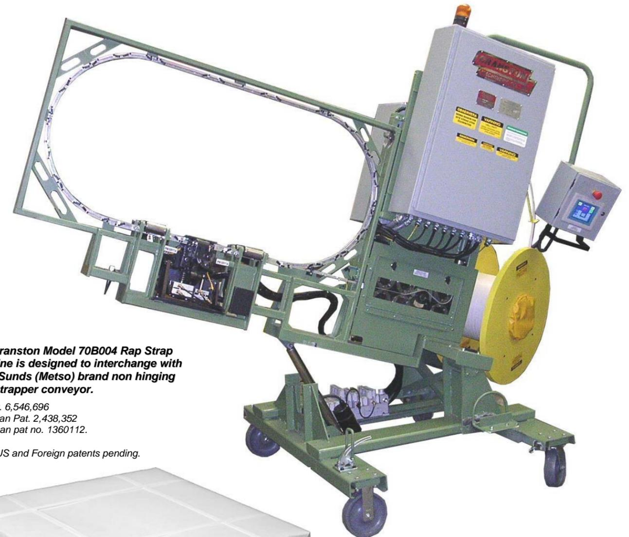
The Cranston Model 70B004 Rap Strap Machine is designed to interchange with most Sunds (Metso) brand non hinging wire strapper conveyor.
