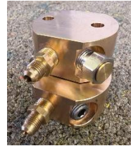
Top cylinder shown with IPRV. Bottom cylinder has Plug.
